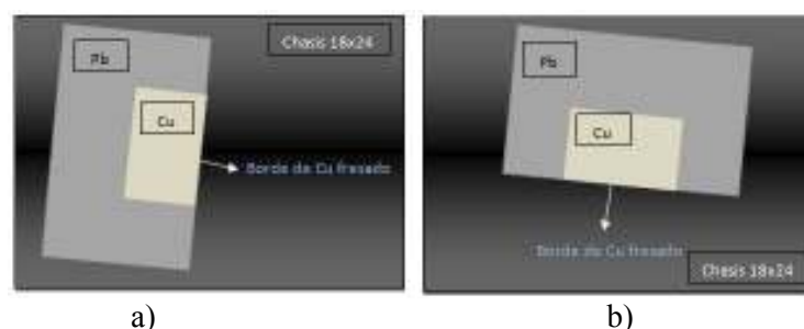
Figure 11. Position of the phantom: a) perpendicular to the axis anode - cathode; b) parallel to the axis anode - cathode.
