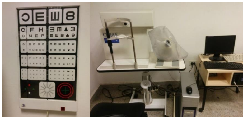
Figure 5. On the left, Snellen chart for VA measure. On the right OQAS System to measure the OSI (Object Scatter Index).
