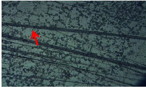
Figure 2. Striped test piece and inoculated with yeast. Notice that the thicker stripes permit yeast housing.
