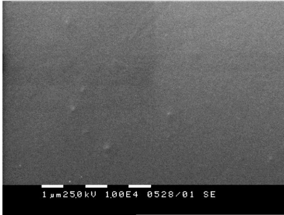
Figure 7. ta-C film implanted with \text{Ga}^+ , D_1 = 3 \times 10^{14} \text{ cm}^{-2} .
