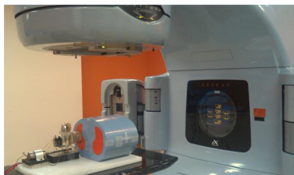
Figure 2. Irradiation technique of the dynamic thorax phantom for both IMRT and VMAT technique.
