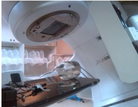
Figure 1. The setup of 100mm pencil ionization chamber in 16 cm diameter CTDI phantom for CBCT head protocol.
