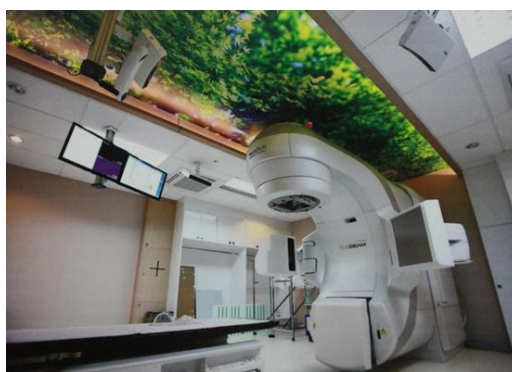
Figure 1. The 3 camera pods of 3D surface tracking system in TrueBeam linear accelerator.
