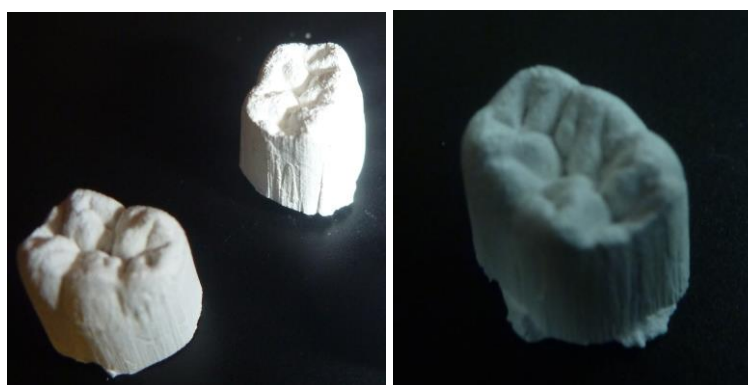
Fig. 6. Three-dimensional dental structure obtained from 3D-model of a human tooth by technology of laser milling.
