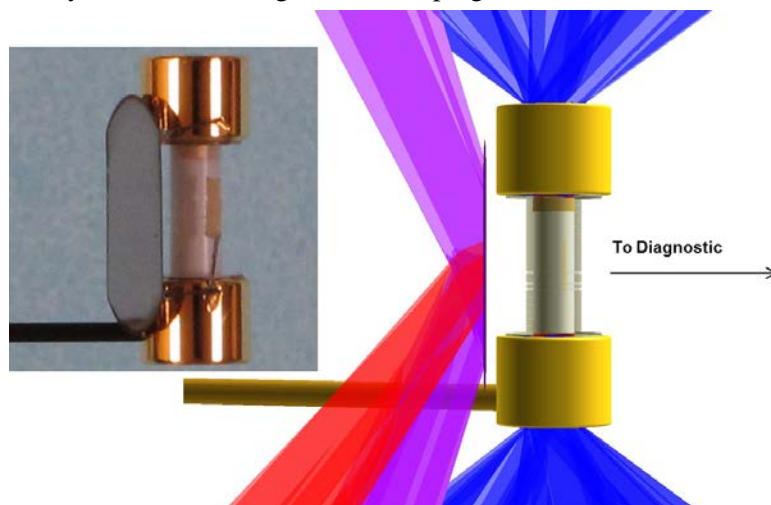
Figure 3. A visual representation of the NIF Shock/Shear setup. The main target (gold) sits at the center of the target chamber supported on a stalk from the left, with halfraums on top and bottom, which are driven by 60 top and 60 bottom outer cone beams (blue beams) with 310 kJ each of the halfraums. Two outer quads (red) and five inner quads (violet) are pointed at the backlighter foil (purple edge-on) driving it with \sim 163 kJ of laser energy to produce the radiograph. (image inset) The target as actually built.
