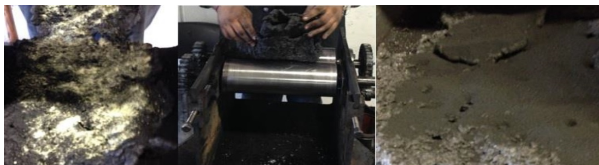
Figure 1. Lamination process of components that conforms the rubber mixtures.
