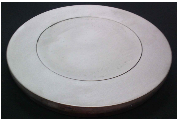
Figure 3. Composite cathode: the inner disc part is formed of mixed titanium and boron powders and the external ring part made of 99.9% titanium.
