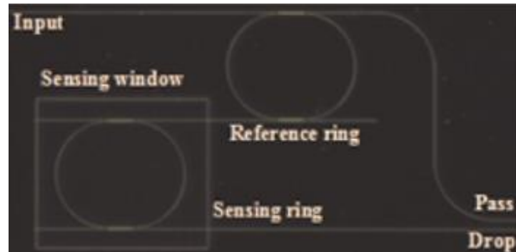
Fig. 1 Optical microscope image of the cascaded double ring sensor based on SOI nanowire.
