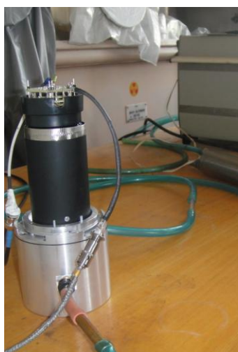
Figure 2. Prototype scintillation detector LABR1.
