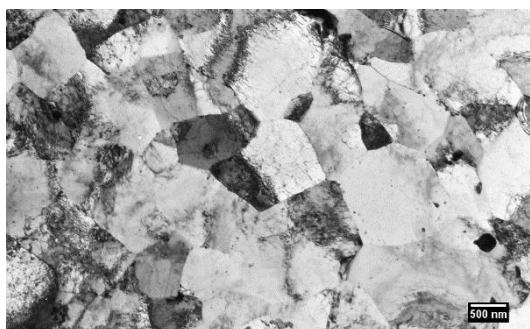
Figure 1. Bright field TEM image of sample KOC 5-3 in as- received state. Microstructure contains polyedric ferritic grains.
