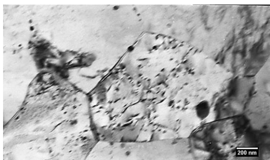
Figure 3. Interaction of dislocations with precipitates in KOC6-3.
