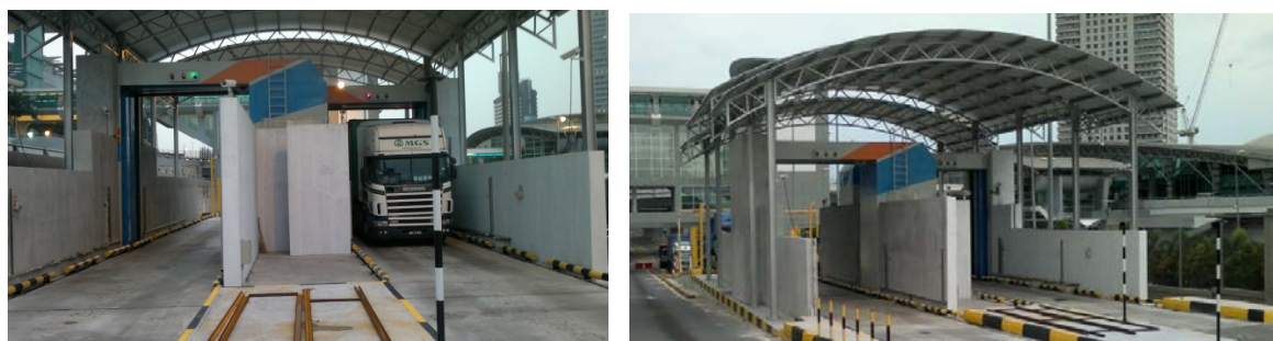
Figure 3. Custom inspection system in Bangunan Sultan Iskandar in BuHit Chaqar, based on two betatrons with energy of 7.5 MeV.
