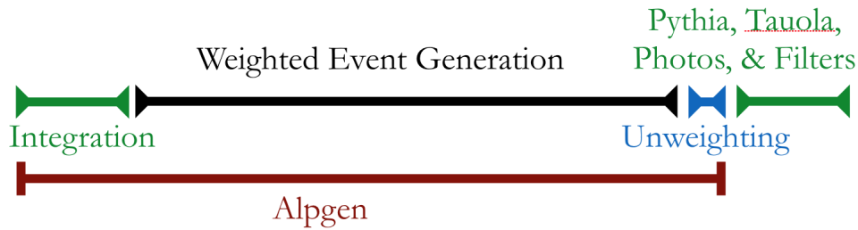
Figure 1. Typical AlpGen workflow running on the grid. Each line segment represents an independent execution step.
