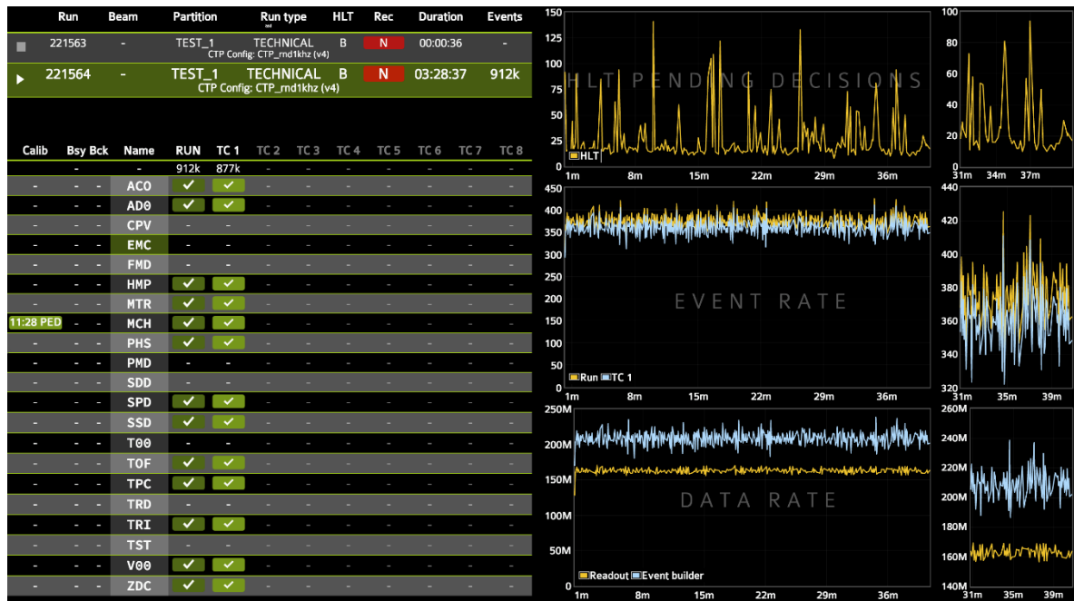
Figure 4. Snapshot of default layout. On the left column, the following widgets are displayed (from top to bottom): Active Global Runs Overview Widget and Detector Status Widget. On the right column, the following widgets are displayed (from top to bottom): HLT Pending Decisions Plot Widget, Event Rate Plot Widget, and Data Rate Plot Widget.
