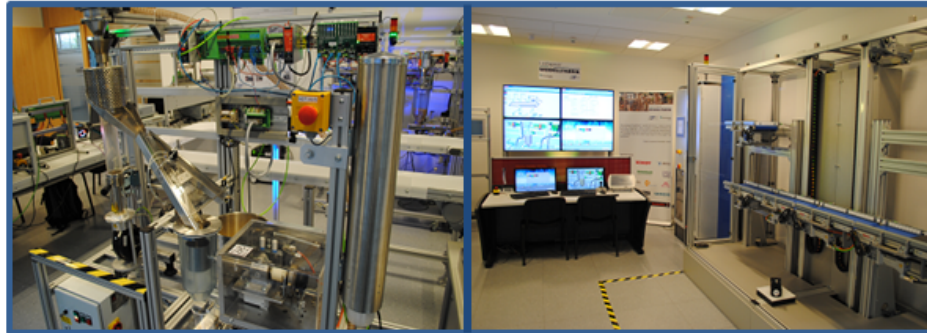
Figure 7. a) Module for bulk goods processing b) Conveying system
