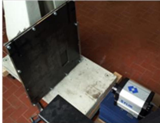
b) specimen lodge and position of the infrared camera
