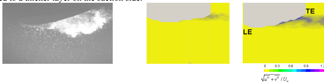
(a) the fluorescent particles in the flow field (b) \alpha=0^\circ, \sigma=0.40 (c) \alpha=8^\circ, \sigma=0.80
