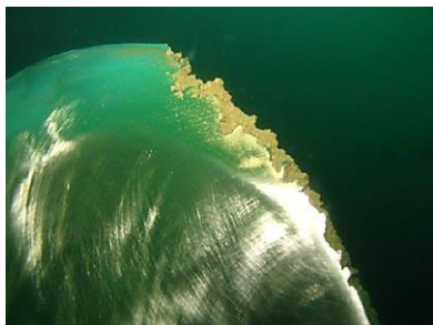
Figure 3. Erosion damage on the propeller.
