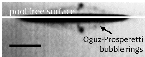
Figure 2. Initial contact I regime. Oguz-Prosperetti bubble rings formed in conjunction with Thoroddsen bubbles ( Fr = 18 , We = 26 ). Frame acquired at t = 0.8 ms after impact. Scale bar = 1 mm.
