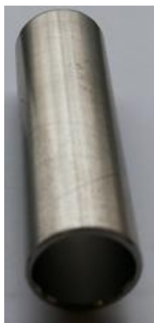
Figure 5. Samples before ion polishing ( \varnothing 9.15 mm)
