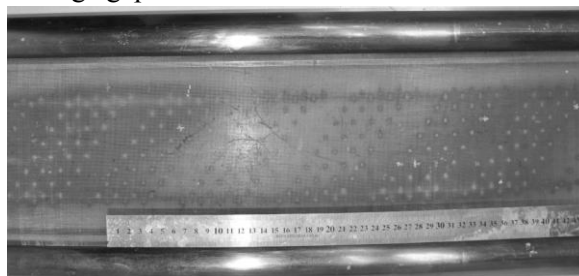
Figure 2. Ion beam autograph left on the emission grid on the side of the high-voltage acceleration gap in the experiment with no mask in the emitter.
