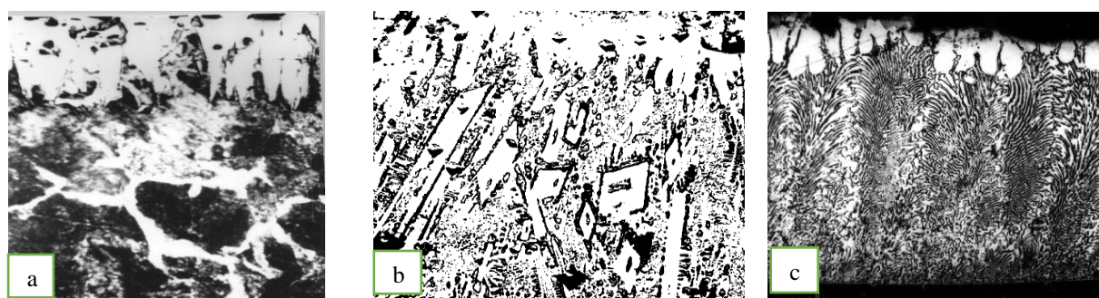
Figure 1. Layers boride microstructure formed on steel 45 surface: solid phase borating (a) and electron-beam boriding - daub from amorphous boron (b) and \text{B}_4\text{C} (c); a - \times 250 , b, c - \times 500
