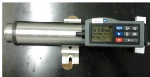
Figure 12. Measurement of roughness on the piece.
