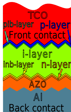
Figure 1. Schematic representation of the cross section of the simulated pin a-Si:H solar cell.
