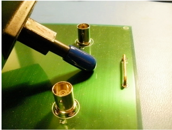
Figure 1. Coupling ESD energy to a PCB.
