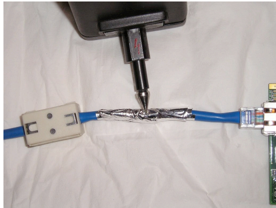
Figure 5. Injecting ESD energy into a cable.
