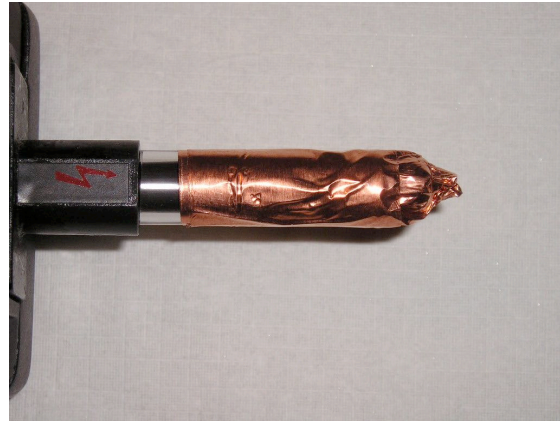
Figure 2. High pass filter on ESD simulator.
