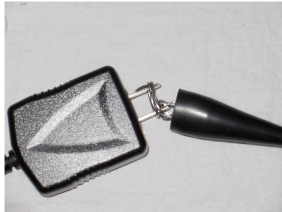
Figure 2. Shorting of the mains connections.
