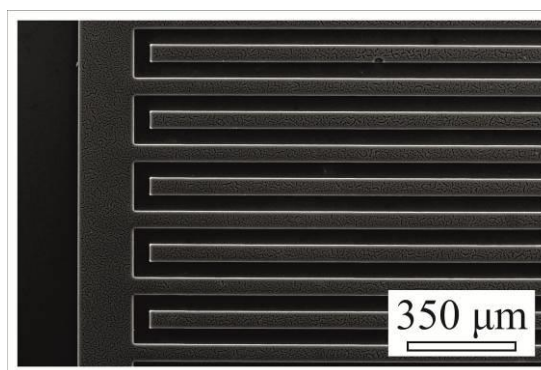
Figure 4. SEM image of planar PsC electrode.
