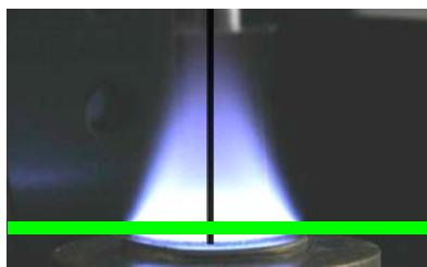
Figure 2. Photo of the studied flame. The black line indicates the area of study, the green line indicates the direction of the laser beam .
