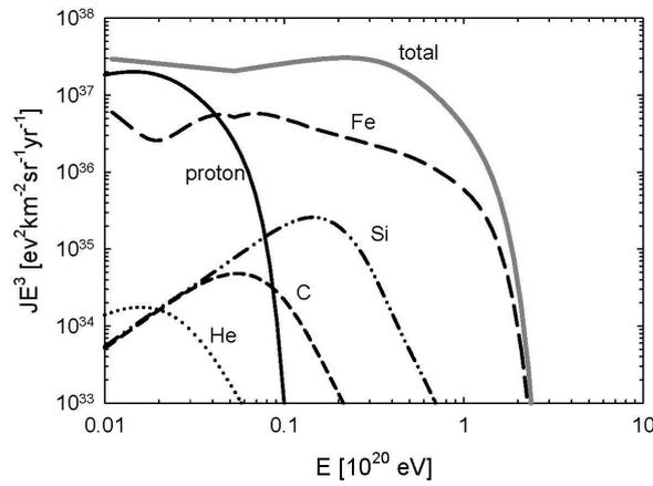
**Figure 3.** Calculated spectra of different types of nuclei for Iron-to-proton source ratio  $S_{Fe}/S_p = 10^{-2}$  and the total observed Auger cosmic ray spectrum at the Earth.
