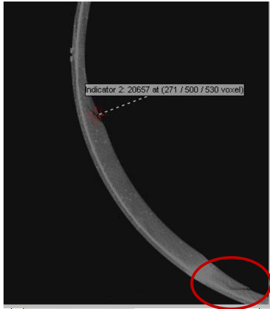
Figure 4. X-ray CT data from post-test inspection of the tube. The image shows a slice through the reinforced section of the tube below the attachment bracket. The red ellipse identifies the damage corresponding to the highlighted regions in figures 4 and 5.
