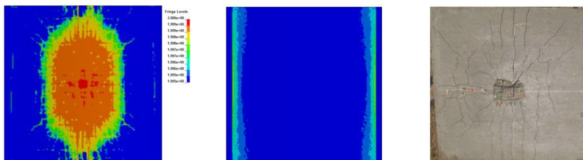
Figure 11. Damage mode of bottom of slab for 0.31 kg, and R = 0.4 m ( Z = 0.59 m/kg 1/3 ). KCC (left), the Winfrith (middle) the experiment [2] (right)
