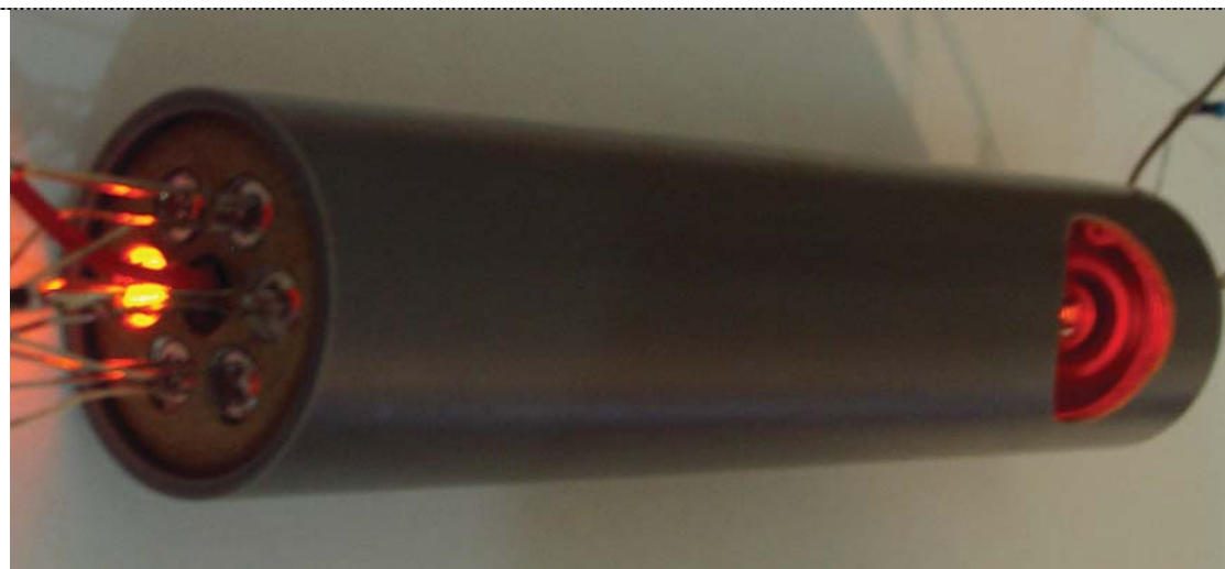
Figure 1. Orange LED is active. Transmitted light illuminates into the photodiode.
