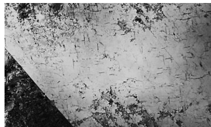
Figure 4. After implantation: Ferritic grain with needle shaped particles.
