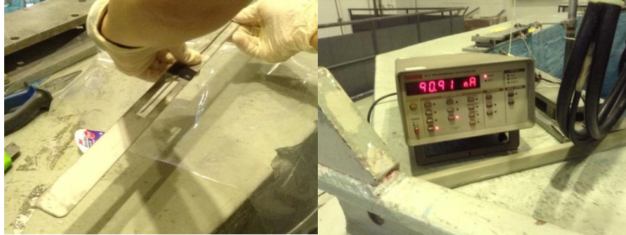
Figure 4. The preparation of SPND and the picoammeter setup.
