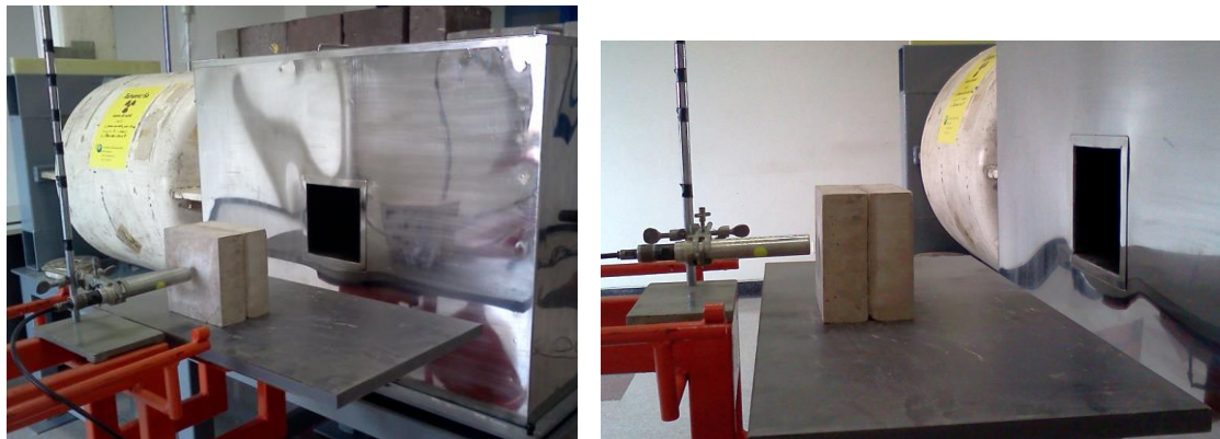
Figure 6. Radiation shielding test setup using Am-241/Be source and \text{BF}_3 detector.
