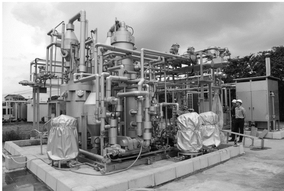
Figure 4. Demonstration plant based on superheated methanol vapor method using bubble column reactor (Designed Productivity: 400 L/d)
