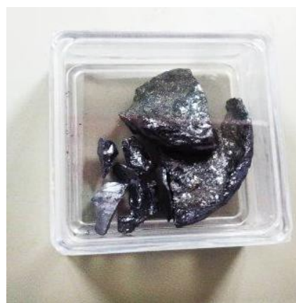
Figure 7. Photo of the obtained Silicon. The impurities level of this sample were 1.1~1.4 ppm for boron and 1.1~2.6 ppm for phosphor.
