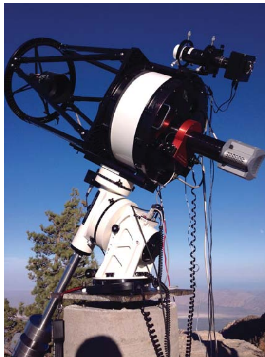
Figure 2. The instrument LOLAS second generation working at the Observatorio Astronómico Nacional at San Pedro Mártir, Baja California in México.
