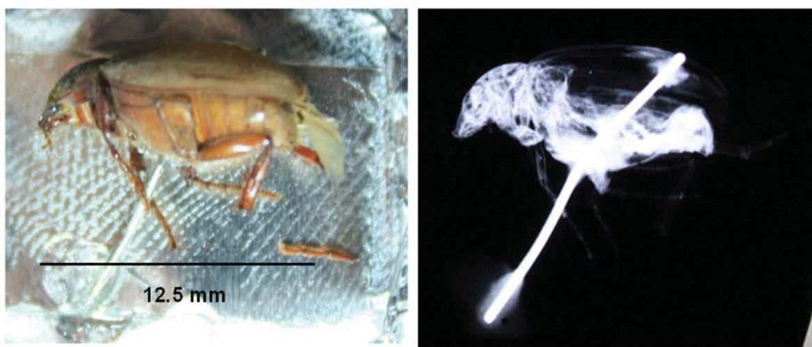
Figure 7: Insect radiography using Tungsten X-pinch of 7.5 \mu\text{m} .
