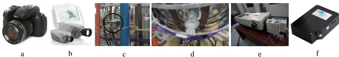
Figure 4. a) Fujifilm camera HS-10 b) Olympus high speed camera ispeed-2 c) Fast photodiode d) Langmuir probe e) Spectrometer THR1000 f) Spectrometer HR4000
