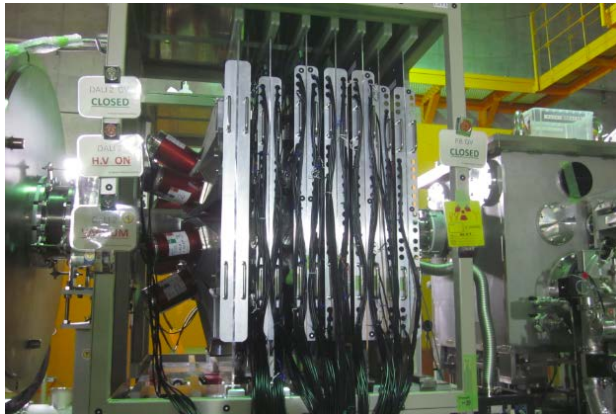
Figure 4: Setup at RIKEN to study \alpha scattering on neutron rich nuclei. The DALI2 array plus additional LaBr detectors measure the \gamma decay from the beam after hitting the liquid He target. The scattered beam particles are measured in the ZeroDegree particle spectrometer.
