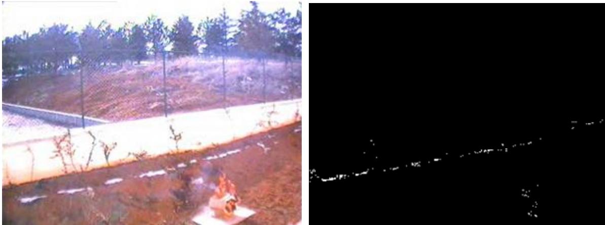
Figure 4. Original snapshot from video (left) and colour filtered image (right).
