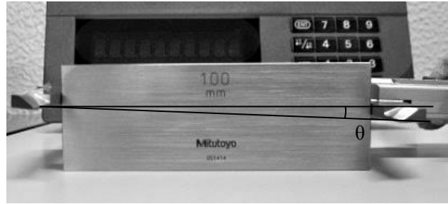
Figure 3. Vertical alignment error
