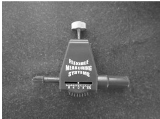
Figure 5. Force control device – made in Flexible Measuring Systems (Denmark)
