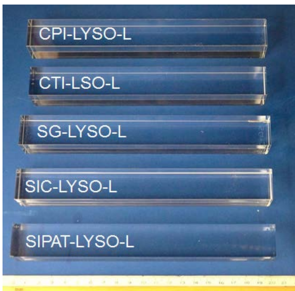
Figure 1. Five 20×20×200 mm 3 LSO/LYSO crystals from CPI, CTI, SG, SIC and SIPAT.
