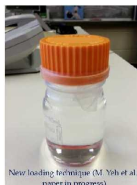
Figure 4. The transparent liquid scintillator.
