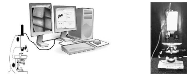
Figure 3. Experimental setup for acquisition and video processing
