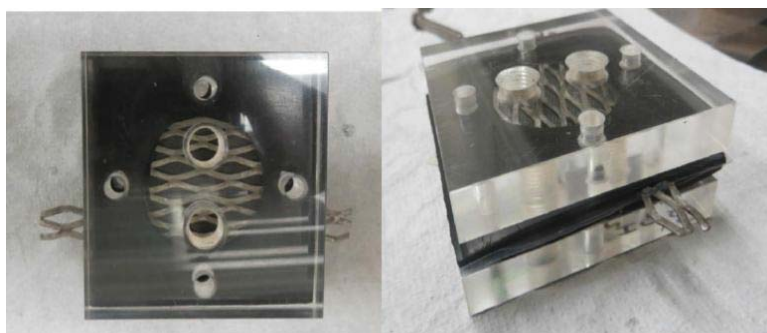
Figure 1. PEM electrolyser construction
